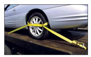
Carriers require chains or straps to prevent the vehicle from moving in any direction.
